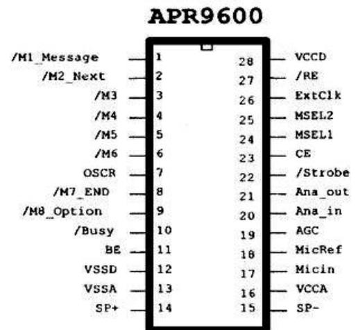
Figure 1 Pin-out of APR9600
