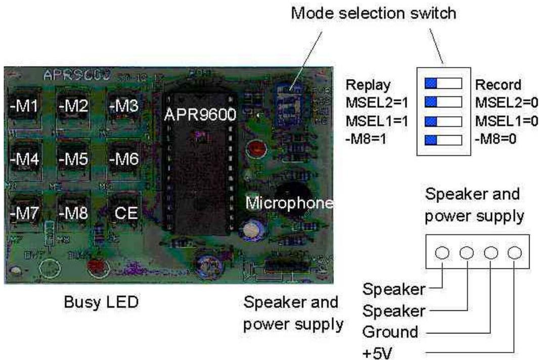
Figure 3 APR9600 module with connector details (to record in parallel mode, the switch setting should be same as displayed above. To record, the top switch should be on the right-hand side. To replay, the top switch should be on the left)
