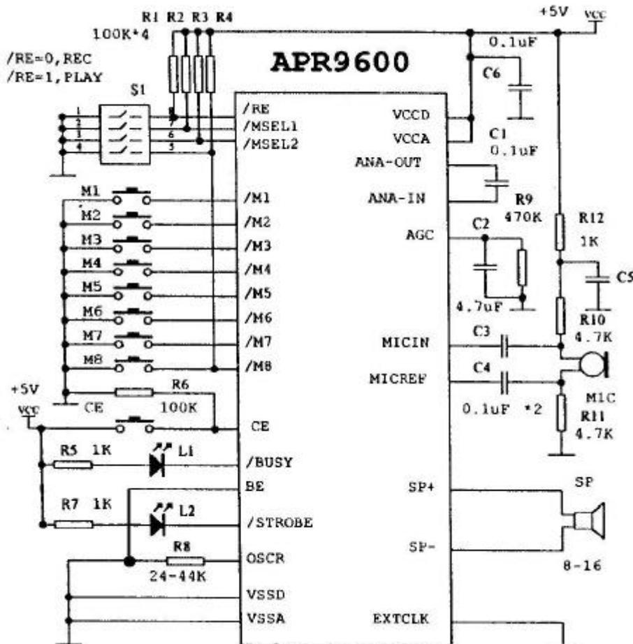
**Figure 2 Typical connections of the APR9600**
