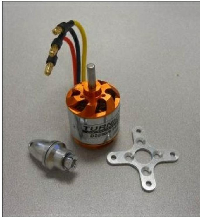
Again, follow the instructions that came with your frame to attach the motor. Then attach the three connections that come from the ESC to the motor.
