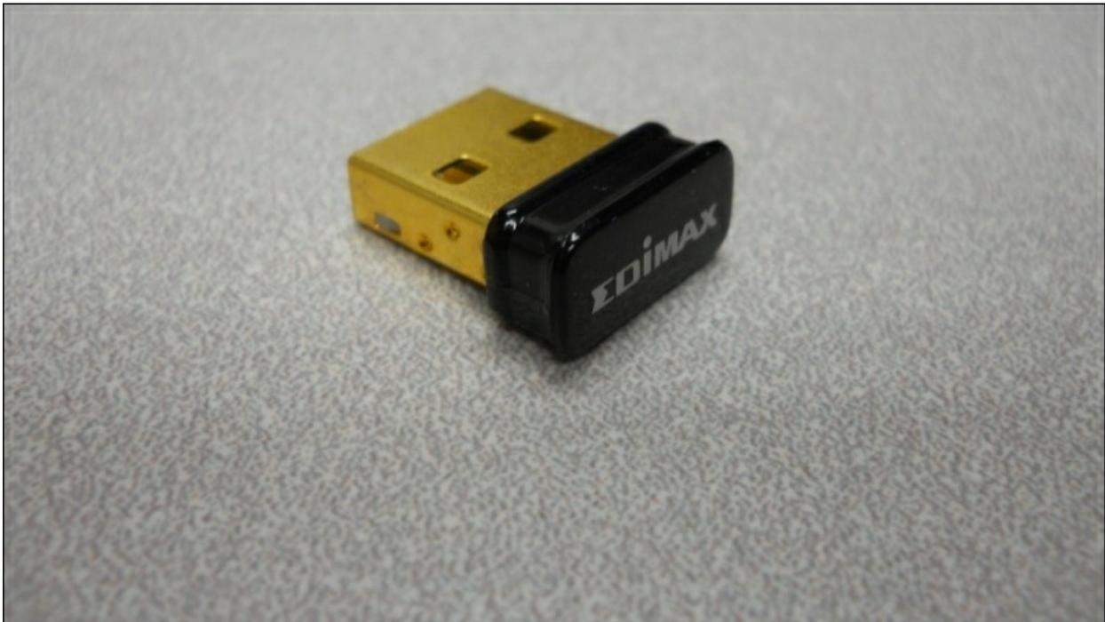
You'll also need to connect a powered USB hub for this process, so that you can access both the keyboard and mouse, as well as the USB wireless LAN device. Now, connect the device to the powered hub.
