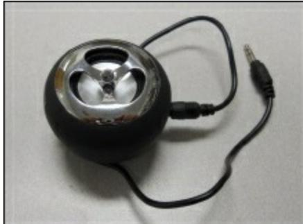
Fortunately, these devices are inexpensive and widely available. Make sure that the speaker is powered because your board will generally not be able to drive a passive speaker with enough power for your applications. The speaker can use either internal battery power or can get its power from a USB connection.
