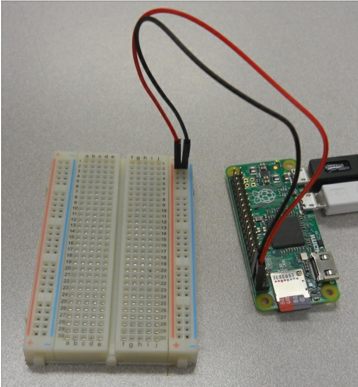
Now you can place the electronic parts on the breadboard. Place the LEDs so that one wire is on one side of the middle split of the breadboard. The direction on the LED is important; make sure that the longer of the two wires is on the left-hand side of the hole.
