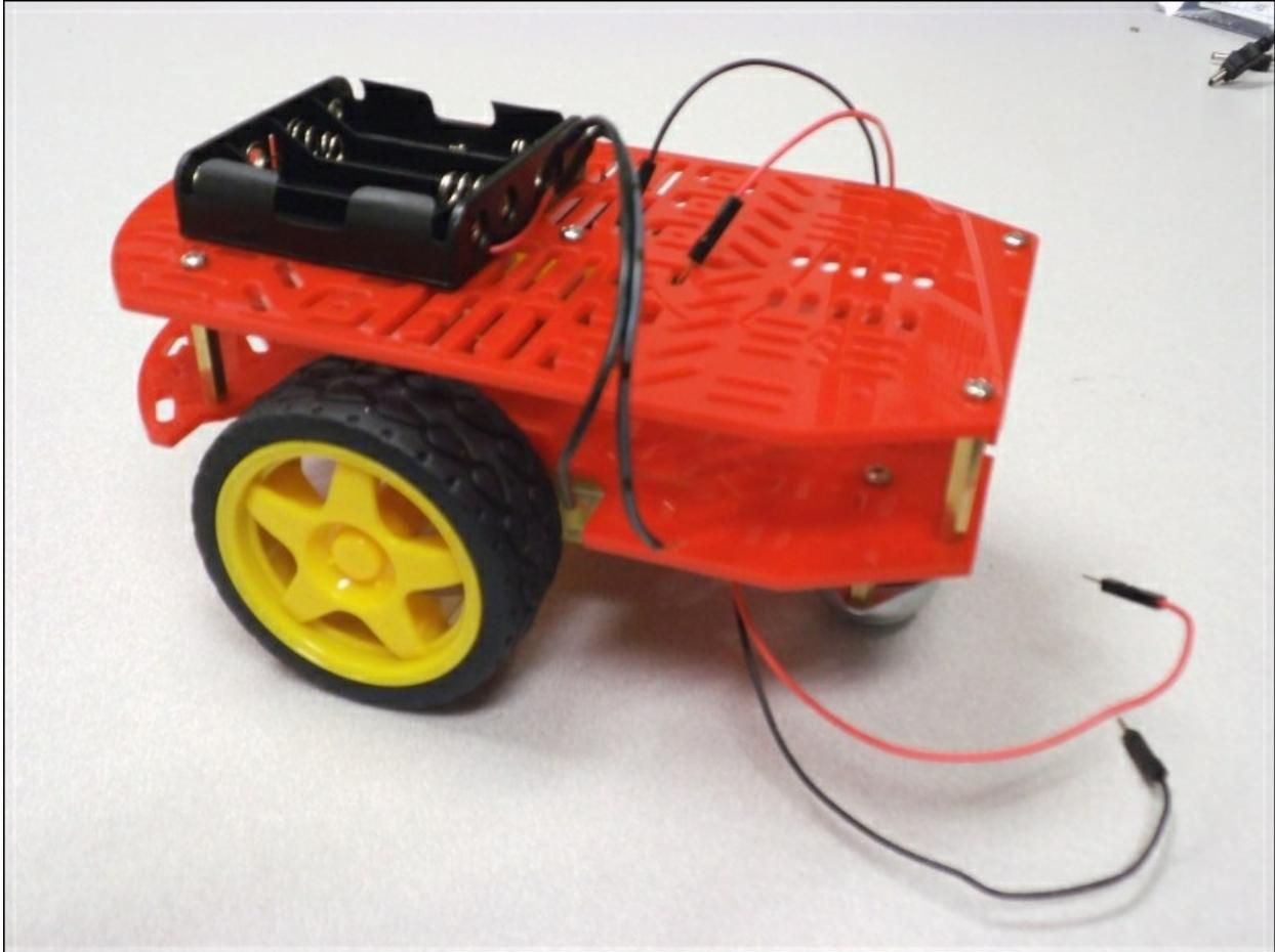
This one also needs to be assembled but it is fairly straightforward. You could also choose a tracked platform instead of a wheeled platform. A tracked platform has more traction but is not as nimble, as it takes a longer distance to turn. Again, manufacturers make pre-assembled units. The following image is an example of a pre-assembled tracked platform made by Dagu. It's called the Dagu Rover 5 Tracked Chassis:
