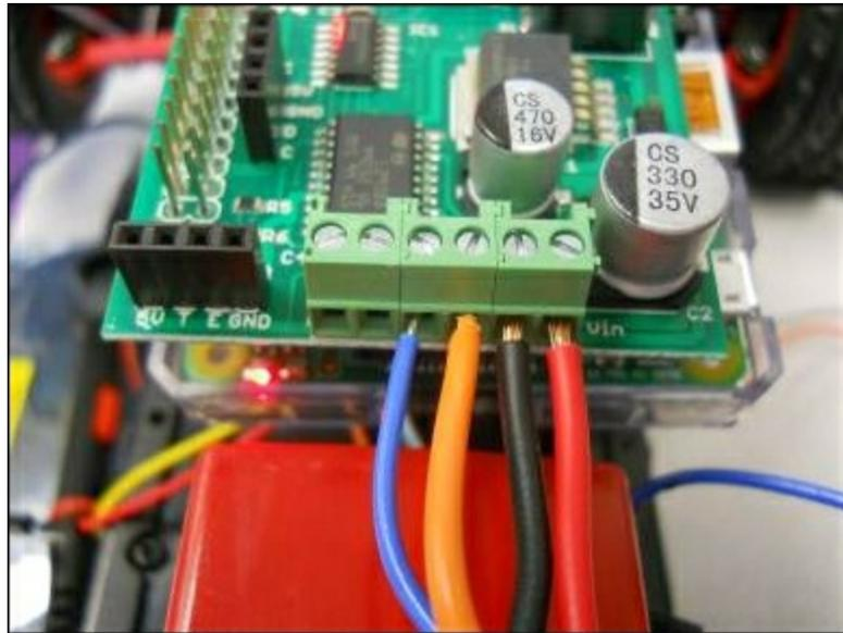
3. Connect the front drive connector to the motor 2 connectors on the board, as shown in the following image:
