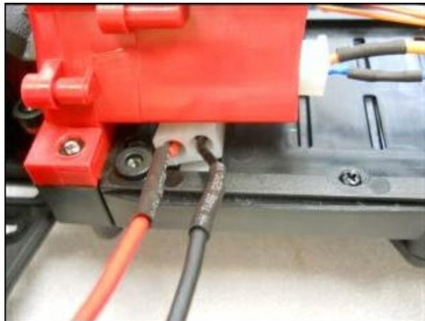
To control the car, you'll need to provide each of the control signals. The + or - 6-volt signals cannot be sourced directly by Raspberry Pi Zero. You'll need some sort of a motor controller to source the signal to control the rear wheel drive of the car and the turning mechanism of the car. The simplest way to provide these signals is to use a motor shield, an additional piece of hardware that is installed on top of Raspberry Pi Zero and can source the voltage and current to power
