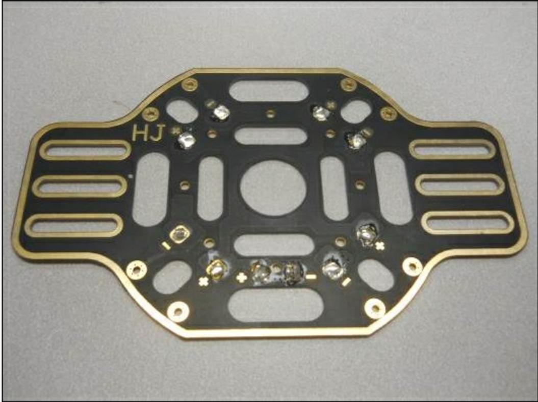
Note the + and – connections; each connection will be soldered to all the ESCs. The following is an image of the motor controller:
