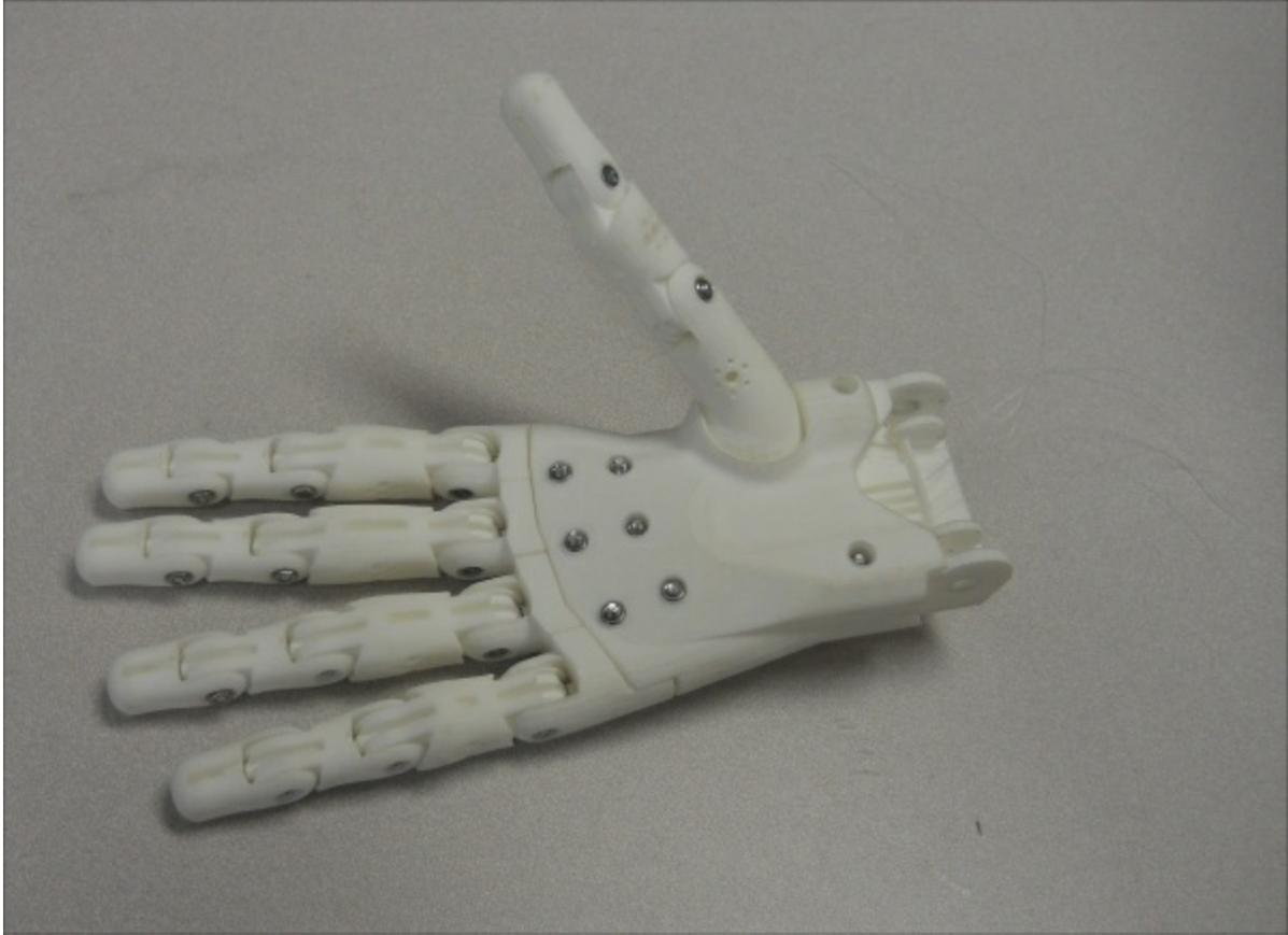
If you have access to a 3D printer, you can also download and print the hand yourself. Here is the link: <https://www.thingiverse.com/thing:288856>. Once you have assembled the hand, you'll need to add the servos to control the hand and the wrist. To control the hand, you'll pull on five separate fishing lines that come out of the hand. Here is an image of those fishing lines:
