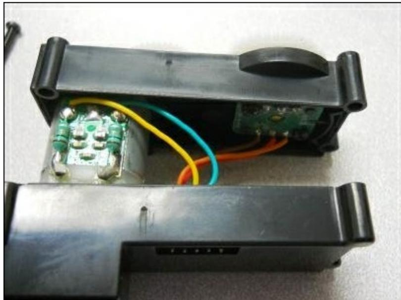
As you can see in the preceding image, the blue and yellow wires are attached to a DC motor, and the orange, brown, and red wires are attached to another control circuit. The motor will drive the wheels left or right, the polarity of the voltage will determine the direction, and its magnitude will cause the wheels to turn more or less sharply. The
