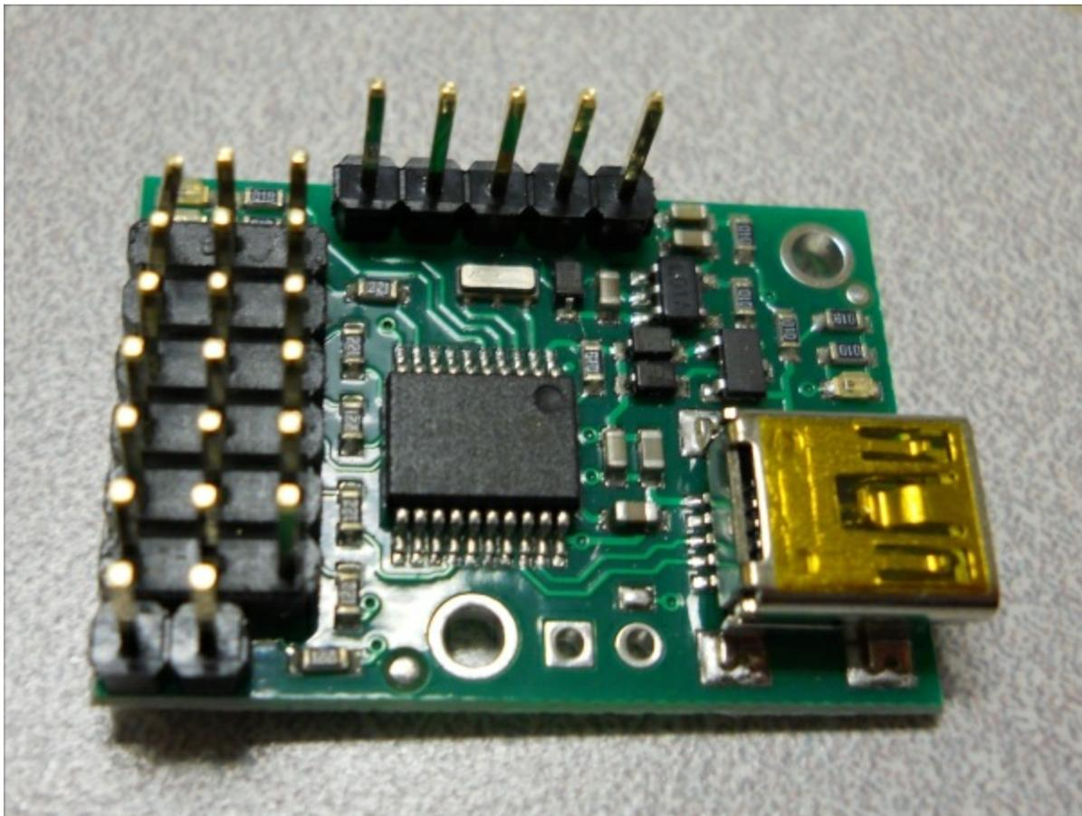
Make sure you order the assembled version. This piece of hardware will turn the USB commands from the Raspberry Pi Zero into signals that control your servo motors. There are two connections that you'll need to make to the servo controller to get started: the first to the
