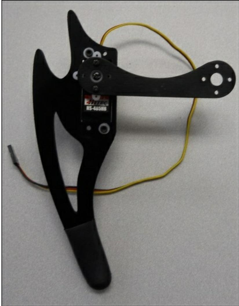
3. Complete the leg by connecting two of the servo brackets together at right angles, mounting the HS-645MG onto one of the brackets, and then connecting this servo to the interconnecting piece, as shown:
