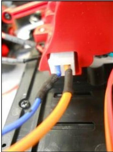
You'll also need to connect the battery power to Raspberry Pi Zero. Here is the modified connection to get the battery power from the car:
