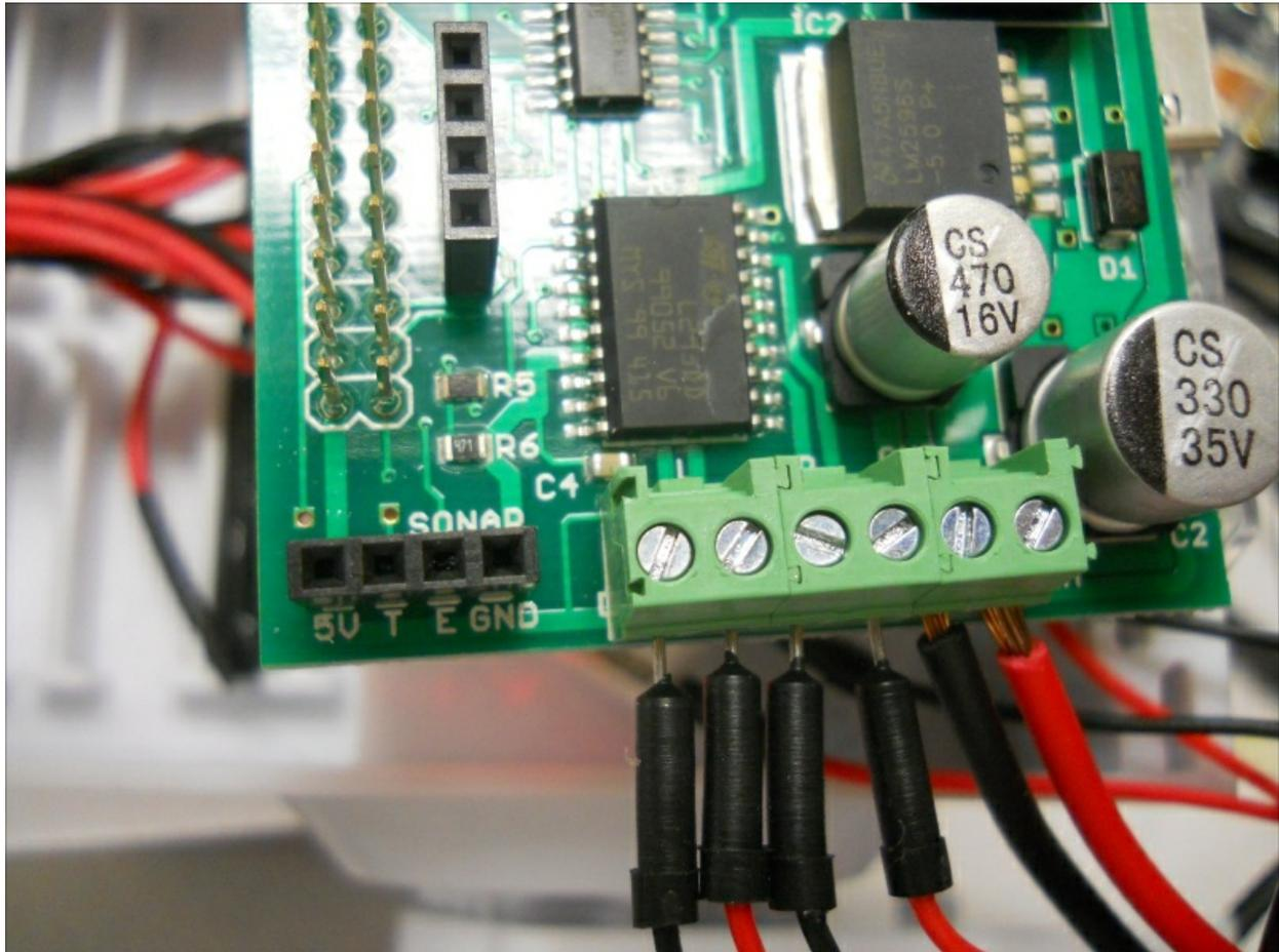
To use this connector, simply connect the VCC to the 5V, the Trig to the T connection, the Echo to the E connector, and the GND to the GND connection. You can then use the library for the motor controller board and simply call the function `rr.get_distance()`. Similarly, there is also a special connector and libraries for the I2C interface, if you want to add the compass to your mobile project.
