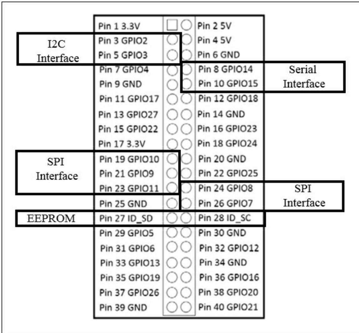
You'll connect the device to pins 1, 3, 5, 7, and 9. For these connections, you'll want female-to-female jumper wires:
