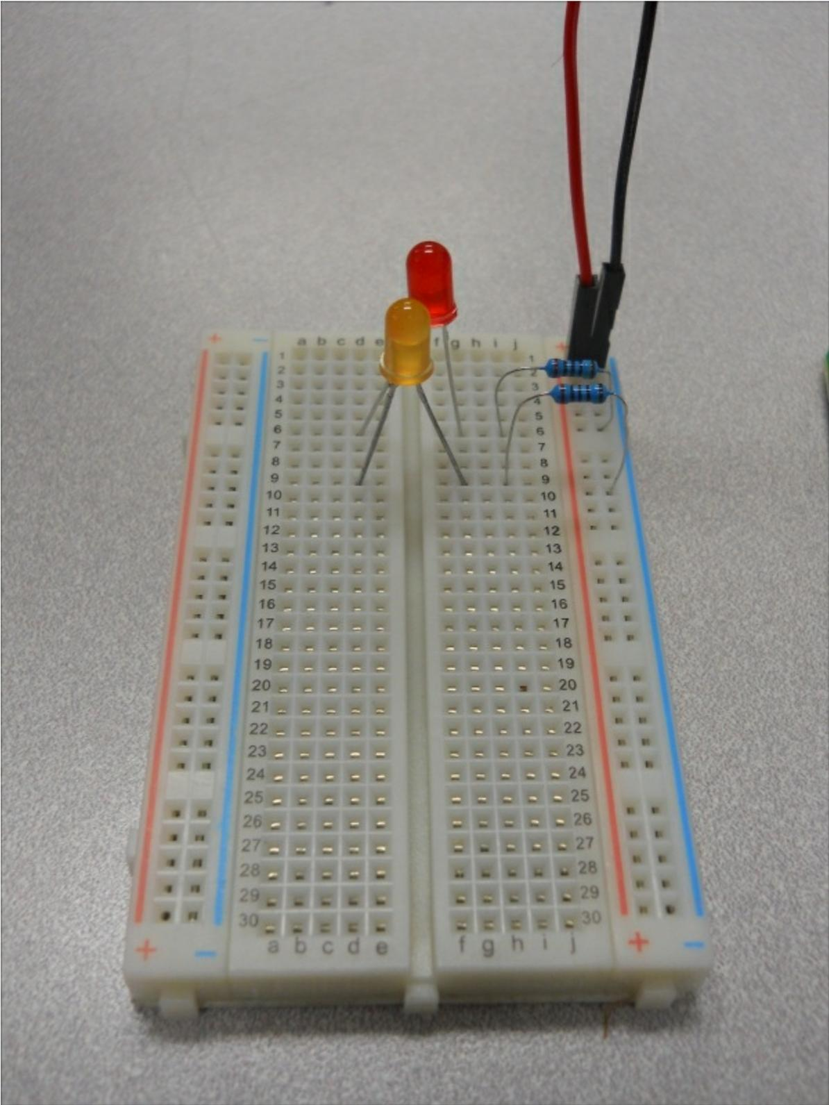
Now you'll use the jumper wires to connect to Raspberry Pi Zero's GPIO pins. You'll connect to pin 13 (GPIO 27) and pin 15 (GPIO 22), as shown:
