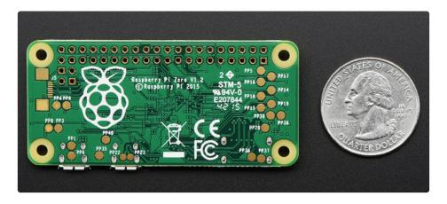
Way smaller than the Pi 2 or B+ and even smaller than the A+, its 60% the size of the A+: same length, and about half the width:
