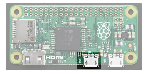
In order to connect a USB device (mouse, keyboard, WiFi) etc you'll need a <u>USB OTG micro B to A cable</u> (http://adafru.it/1099):
