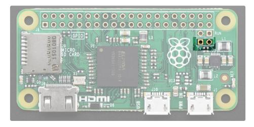
The hole on the left, nearest to the **TV** text, is the signal (+) line, the pin to the right of it is the ground (-) line. Solder two wires to these pads and connect them to an <u>RCA Jack</u> (http://adafru.it/2792) like this one
